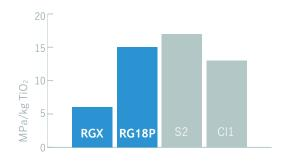
Comparison of the optical properties of **PRETIOX** titanium dioxide grades with sulphate /S/ and chloride /Cl/ competitive samples in grey LDPE films.
